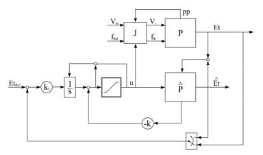
Fig. 2. Structure of the controller with patient (P), observer ( $\hat{p}$ ), state feedback control vector (k), additional integral part (kI), peak expiratory pressure (pp), measured (Et), observed ( $\hat{E}t$ ) and reference (EtRef) end-tidal CO2 concentration, algorithm block (J) with additional inputs from the anaesthetist (fRd) and (Vtd).
