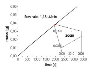
Fig 1. Flow rate of a silicon capillary (no 37) at 500 hPa. .and 22°C.
