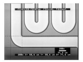
**Fig. 1:** The microchannel is located on the front side of a silicon chip and covered with a pyrex glass wafer (sectional microscope view, 200x).
