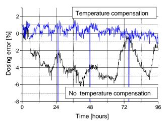
Fig. 2: Compensation for the dosing error of water due to temperature variation.
