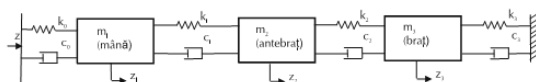
Fig. 1 A simplified linear mechanical system of hand-arm assembly with three degrees of freedom
